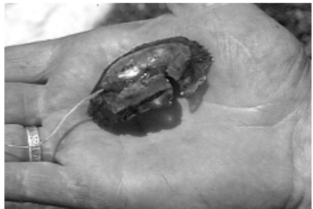
Figure 4. Cracked transmitter package found on the highway.
