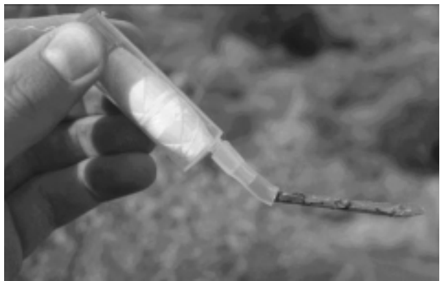
Figure 2. The described thread-trailing device, showing the flexible hinge between plastic stick and syringe with cocoon.
